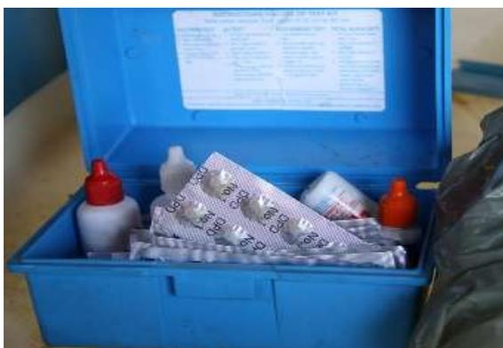
*HTH swimming pool kit with DPD reagents was used to determine free chlorine concentrations*
