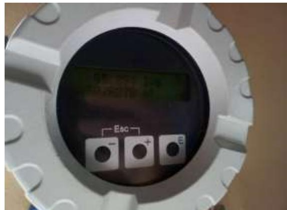
*An inflow measuring device is in place and readings are recorded*
